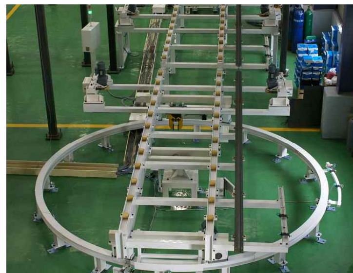
* Cross Transfer in the pit KMC H-1 (Shop test)
